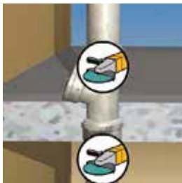
Cut the existing branch just above the slab
