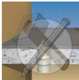
Break the former pipe parts included in the slab
