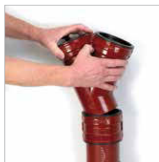
Push the second pipe or fitting into the gasket again ensuring that the spigot is abutted against the central register.
