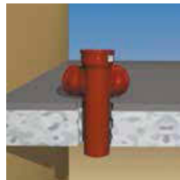
Insert the new branch long tail into the slab
