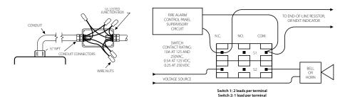
NOTE: The above diagram shows a connection between the common terminal (yellow – S1 and yellow-with-orange stripe – S2) and the normally closed terminal (blue – S1 and blue-with-orange stripe – S2). In this example, the indicator light and alarm will stay on until the valve is fully open. When the valve is fully open, the indicator light and alarm will go out. Cap off any unused wires (e.g. brown with orange stripe).
