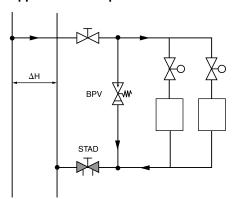
In installations with radiator valves, in which many of the radiator valves have closed, a big part of the pump head will affect the valves since the pressure drop in pipes and accessories has decreased. If the available differential pressure is higher than 30 kPa, noise may occur.
