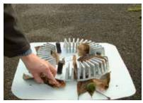
Ensure the leafguard grid is in place. Clean the leafguard grid.
