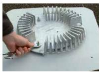
Unscrew the nuts and lift the leafguard grid to remove it.
