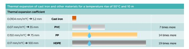
For cast iron, the bracketing system is designed to only carry the weight of the pipe and its content, which makes the designers' work easier. Plastic pipes, however, expand considerably with increasing temperature. Their bracketing system must be designed and adapted accordingly, as it can significantly affect the pipework's stability and performance over time.
