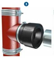
3. Mark the insert depth on the connecting pipe. Apply a lubricant and push in. The assembly is complete.
