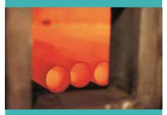
The spun pipes are placed and rotated in a heat treatment furnace at 950°C and then gradually cooled again. This step is essential to the process as it transforms the cast iron's metallurgical structure.
