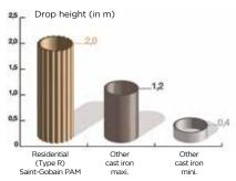
The test consists of dropping a mass of 2.75 kg on a descent at increasing heights until it breaks or cracks.
