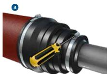
1. Push the open end of the PAM MULTIQUICK connector over the pipe end and place the hose clamp to its tightening position.
