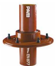
The roof penetration device is a set of two ductile iron flanged fittings – one of the flanges is fixed, the second is movable – equipped with rubber gaskets. Rubber gaskets are available in EPDM or NBR quality where hydrocarbons may be present.
