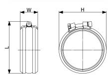
The PAM Rapid is designed for full tightening with "zero gap", there is no need to check the torque. For DN 250 and 300, apply the following torque:  $25 \, \text{N.m.}$
