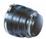
To connect PAM cast iron pipes with an outside diameter of 109-112 mm (tolerance range for PAM cast iron pipes is DN 100) to other rigid materials with an outside diameter from 72-110 mm. To connect PAM cast iron pipes with an outside diameter of 109-112 mm to waste pipes with an outside diameter up to 115 mm maximum. The connection is made with two hose clamps both suitable to address larger diameter tolerances.
