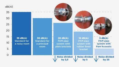
Tests according to standard NF EN 14366 (IBP laboratory). For a flow rate of 2 liters/second, wall:  $220 \text{ kg/m}^2$ .
