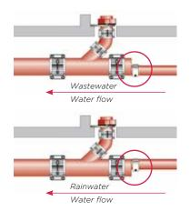
The internal diameter of pipes cannot be reduced in the direction of the water flow, except in the case of pipework operating at full bore, under negative pressure such as in the EPAMS siphonic roof drainage system. The addition of branch connections, or changes of fall liable to increase the water flow rate, may require an increase in internal pipe diameter. This increase can be applied upstream of the new branch connection, using a tapered pipe (see p.90).
