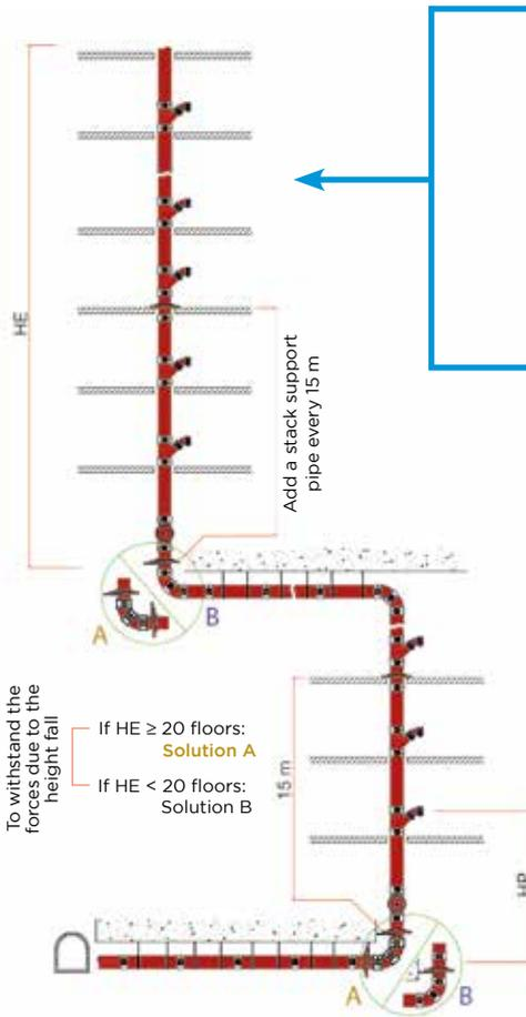
To withstand the forces due to the height fall
