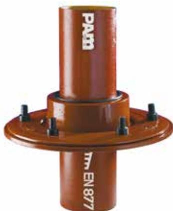
The roof penetration device is a set of two ductile iron flanged fittings - one of the flanges is fixed, the second is movable - equipped with rubber gaskets. Rubber gaskets are available in EPDM or NBR quality where hydrocarbons may be present.
