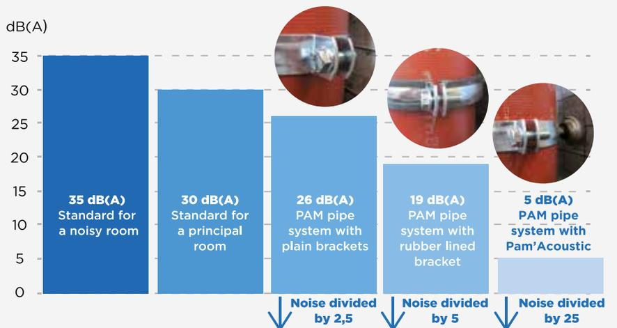
Tests according to standard NF EN 14366 (IBP laboratory).
