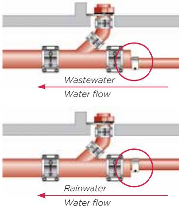
The internal diameter of pipes cannot be reduced in the direction of the water flow, except in the case of pipework operating at full bore, under negative pressure such as in the EPAMS siphonic roof drainage system. The addition of branch connections, or changes of fall liable to increase the water flow rate, may require an increase in internal pipe diameter. This increase can be applied upstream of the new branch connection, using a tapered pipe (see p.90).
