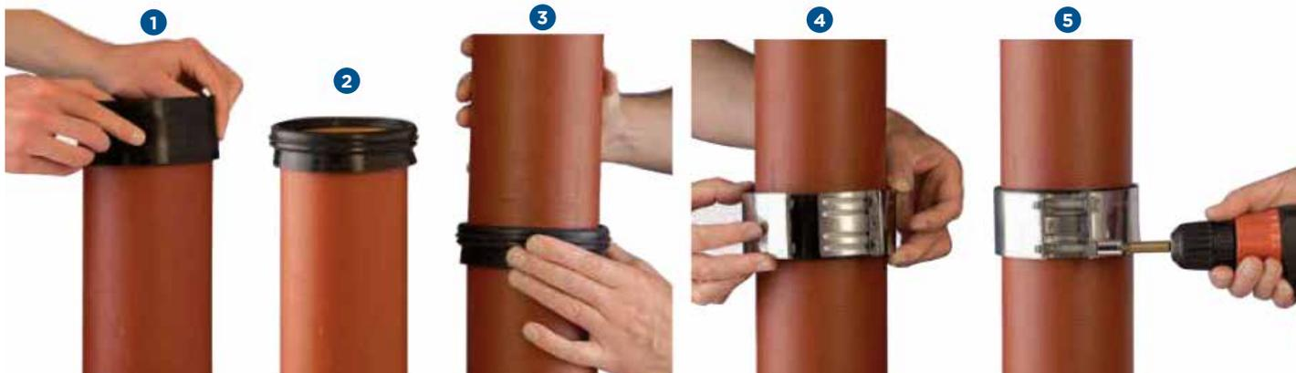
1 *Push the supplied sealing gasket on to the pipe spigot so it abuts the gasket central register.*
