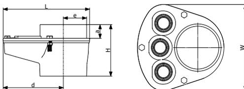
The multi-waste manifold simplifies waste plumbing by grouping all associated pipework from various sources such as sinks, basins, bidets, urinals and showers to one internal point above the finished floor level.
