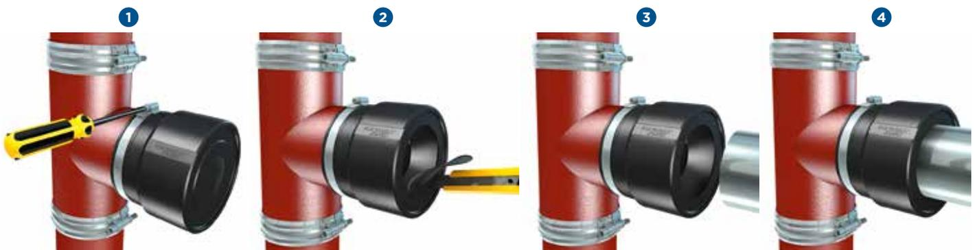
1. Insert the PAM KONFIX rubber connector loosely onto the pipe until the stop point is reached. Then secure to the pipe by tightening the hose clamp screw.
