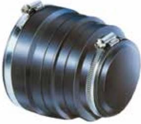
To connect PAM cast iron pipes with an outside diameter of 109-112 mm (tolerance range for PAM cast iron pipes is DN 100) to other rigid materials with an outside diameter from 72-110 mm. To connect PAM cast iron pipes with an outside diameter of 109-112 mm to waste pipes with an outside diameter up to 115 mm maximum. The connection is made with two hose clamps both suitable to address larger diameter tolerances.
