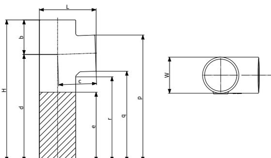
"All dimensions are in mm and nominal weights are in kg" - "Hatch patterned area in the drawings shows the max. cutting length".
