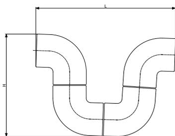
TRAPS DN > 250: Installation with 88° bends
