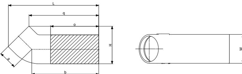
"All dimensions are in mm and nominal weights are in kg" - "Hatch patterned area in the drawings shows the max. cutting length".
