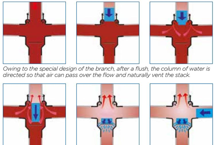
*Owing to the special design of the branch, after a flush, the column of water is directed so that air can pass over the flow and naturally vent the stack.*
