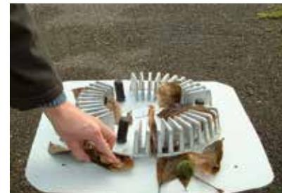
*Ensure the leafguard grid is in place. Clean the leafguard grid.*
