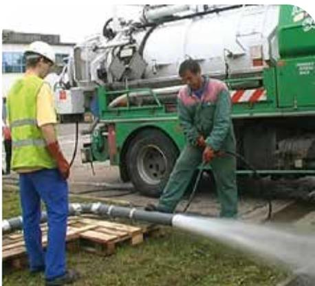
The S and Plus ranges, assembled and anchored, have successfully passed a high-pressure jetting test: cleaning pressure of 120 bar from the pump, which means 100 bar at the nozzle outlet, without leaks or misalignment.
