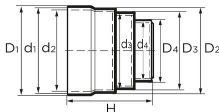
The Multiquick connector DN 100x70 allows connections between other materials with an outside diameter from 72 to 110 mm, to our cast iron range DN 100 with a maximum outside diameter of 115 mm. There are several pre-cut options. EPDM and hose clamp made of chrome steel no. 1.4016.
