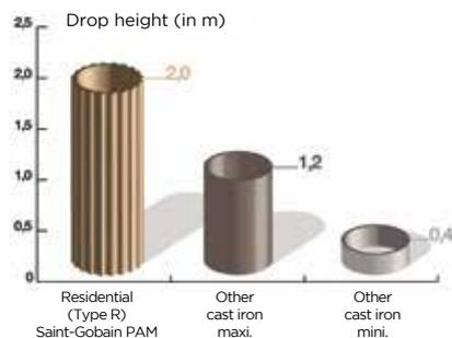
The test consists of dropping a mass of 2.75 kg on a descent at increasing heights until it breaks or cracks.
