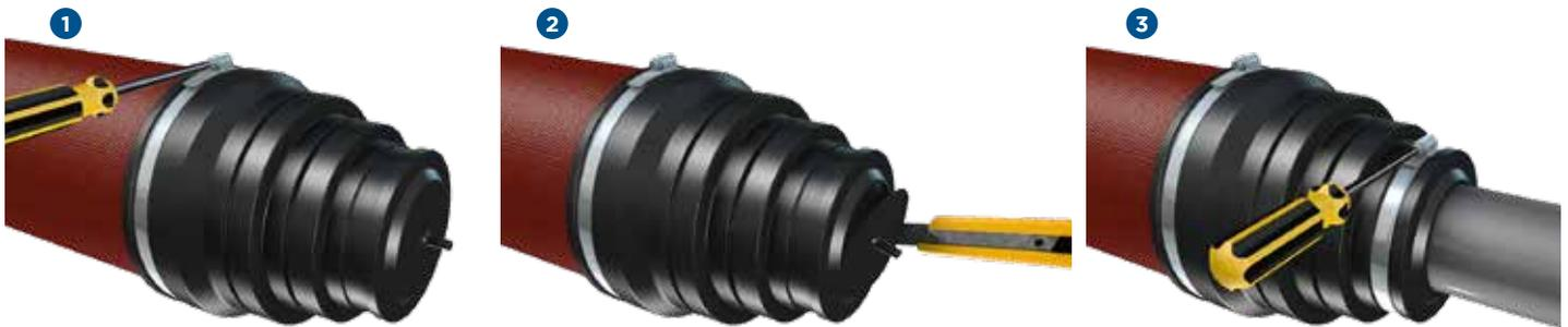
1. Push the open end of the PAM MULTIQUICK connector over the pipe end and place the hose clamp to its tightening position.
